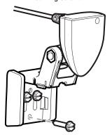
3. Re-position the transducer assembly against the transom of the boat, then hand install the first three screws (two on the outside edges and one in the 3rd mounting hole). Make sure that the transducer location and the pivot angle have not changed, then fully tighten all three mounting screws. Hand-tighten only!
